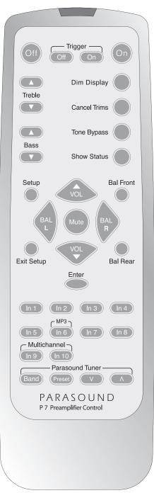
**Dim Display Button** – Each press of the Dim button decreases the brightness of the front panel display tube, the buttons and P badge illumination. After pressing the Dim button 4 times the front panel display tube will go completely dark. In this mode the display will remain completely dark until any button on the remote or front panel is pressed. The display will then turn back on at a dim setting.
